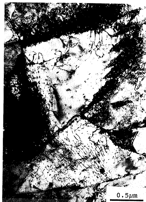
Fig. 10. Widmanstätten ferrite saw-teeth with low dislocation densities and copper precipitates in a copper-containing HSLA steel cooled at 0.1°C/s (from Ref. 27)). TEM micrograph.
