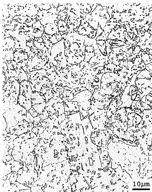
Fig. 13. Granular ferrite formed by continuous cooling of a modified-A710 steel (composition in text) at a rate of 1°C/s. (Courtesy of B. Kloberdanz, Colorado School of Mines) Light micrograph.
