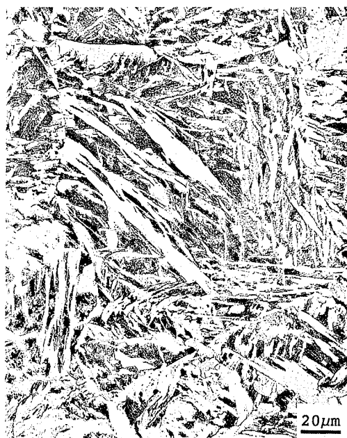
Fig. 9. Widmanstätten ferrite (large elongated white grains) formed in HSLA-80 steel isothermally transformed for 100 s at 600°C. Dark areas are martensite formed during quenching after isothermal hold. Light micrograph. (Courtesy of M. Kumar, Colorado School of Mines)
