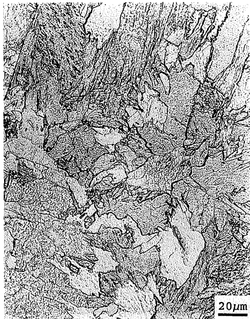
Fig. 11. Quasi-polygonal ferrite formed in ultralow-carbon steel containing 0.005 C and 3 Mn cooled at 50°C/s. (Courtesy of C. C. Tseng, Colorado School of Mines) Light micrograph.
